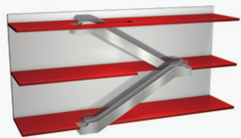
Continuous arrangement (one-way traffic)
